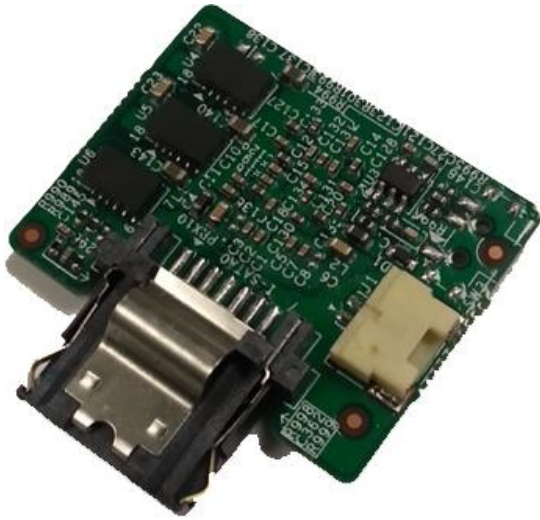
Figure 2-7 (SATADOM) SATA Disk on Module Device
